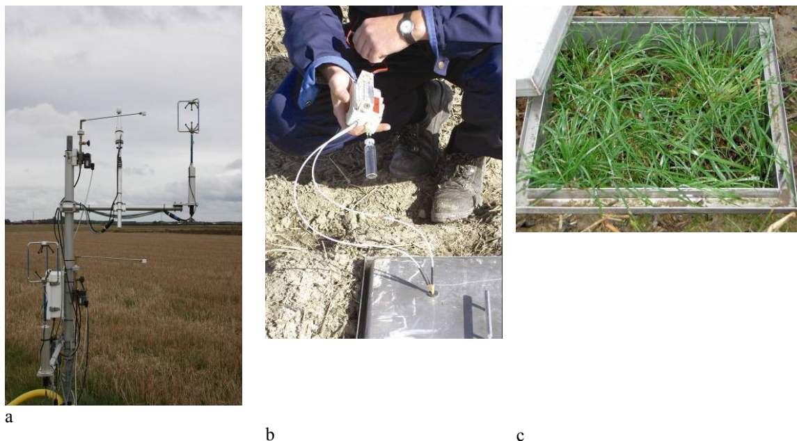
Figure 1. Micrometeorological equipment at Lanna (a), and chambers (b and c) used for gas sampling in the long-term experiment.
